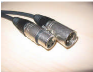
Fig. 7b – XLR Cable, male (right) and female (left) ends shown (female is what will plug into your mixer's output)
