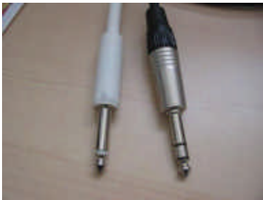
Fig. 7a – 1/4" Cable, also known as TS (left) or TRS (right)
