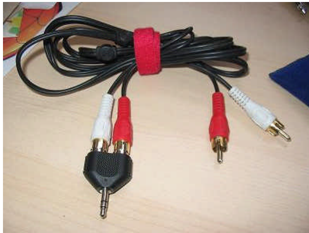
Fig. 7 – 1/8” - Stereo RCA cable made using adaptors
